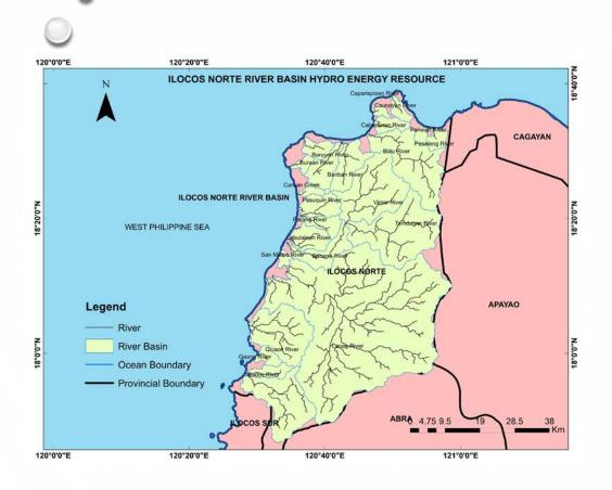
The study was aimed to use remote sensing data particularly Synthetic Aperture Radar (SAR) and Geographic Information System (GIS) technologies to assess the hydroenergy resource potential of Ilocos Norte river basin. Moreover, the study was aimed to delineate river reaches, simulated flow, detect suitable head locations and identify potential locations for possible establishment of hydro-energy power plants.
